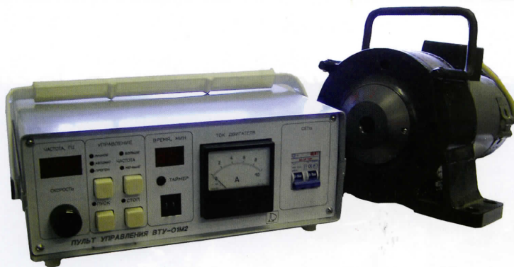
Fig. 3. Overall view of equipment for low-frequency vibratory stress relief
